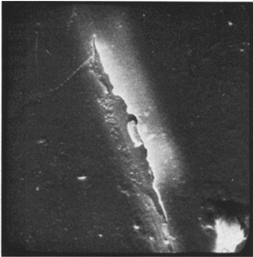
Figure 16 GFRP sheet weathered outdoors at Ottawa for 880 days ( \times 1300 ).
