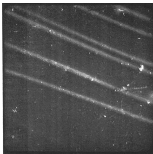
Figure 4 GRP sheet aged for 12 cycles in the Weather-Ometer ( \times 360 ).
