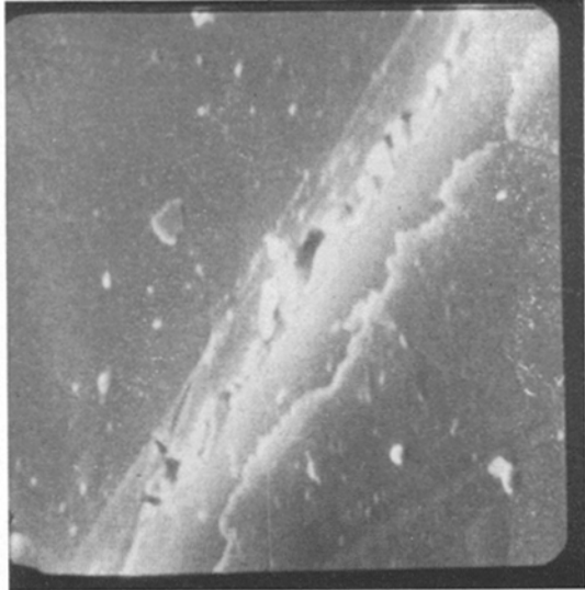
Figure 6 GRP sheet aged for 15 cycles in the Weather-Ometer ( \times 2900 ).
